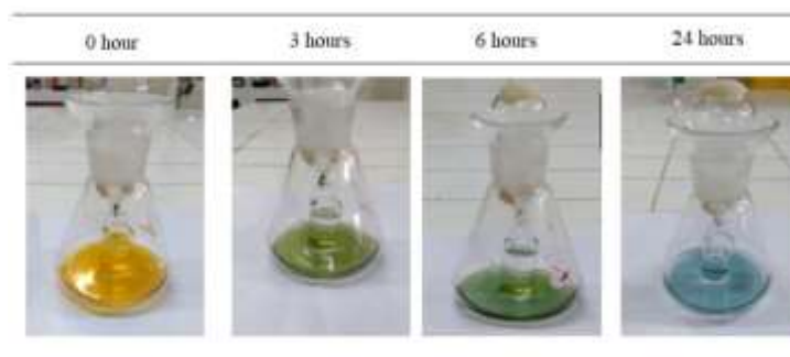
Figure 3. The color change of K_2Cr_2O_7 reagent by standard ethanol 5% in various times.
