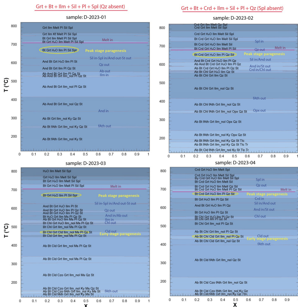
Figure 4. T-X diagrams for predicted phases by GeoPS model on the four Dorbeh metapelites bulk rock composition. Yellow ellipses applied for showing early stage (P1), and peak stage (P1) position. Additionally, phases in/out temperature are determined and melt-in paragenesis is detected as maximum temperature estimation.
