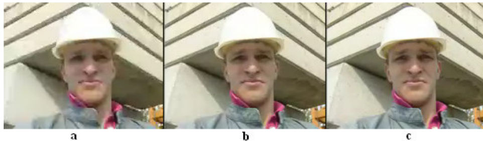
Figure 2. Comparison of transferring video over different paths. a(1 path 80 kbps, PSNR 32.5 dB), b(3 paths 187 kbps, PSNR 36.2 dB ), c(6 paths 278 kbps, PSNR 38 dB).
