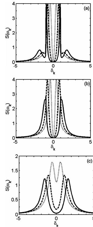
**Figure 5.** The spontaneous emission spectrum  $S(\omega_k)$  (in arbitrary units) for transition from the upper level  $|2\rangle$  to the lower level  $|0\rangle$  as a function of detuning  $\delta_k$  for different reservoirs. a) Double-band isotropic PBG reservoir, b) double-band anisotropic PBG reservoir, c) free vacuum reservoir.  $\Omega = 1.5$  (solid lines),  $\Omega = 1.0$  (dashed lines),  $\Omega = 0.5$  (dotted lines). The other parameters used are the same as those in Figure 2.
