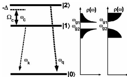
**Figure 1.** Schematic diagram of a three-level driven atomic system. The solid two arrow line denotes the coupling laser, the thin dashed arrow denotes the coupling to the modified reservoir (PBG) and the thick dashed arrow denotes the coupling to the free space reservoir.
