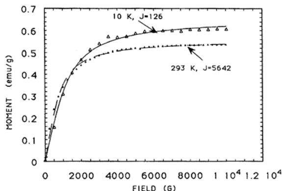
Figure 4. The superparamagnetic contribution to the magnetisation of the Specimen B at 293 K and 10 K obtained as for the Specimen A.
