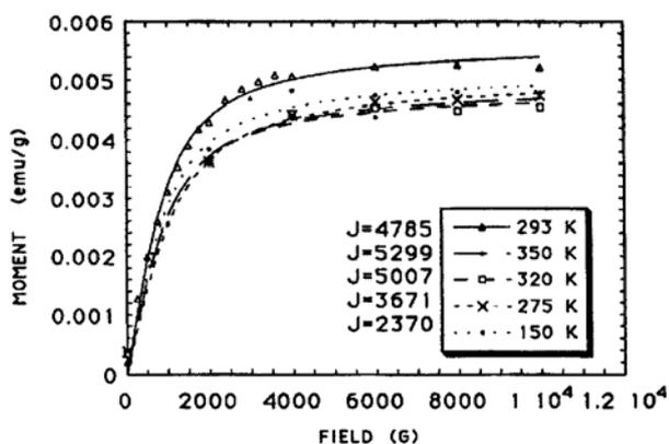
Figure 3. The superparamagnetic contribution to the magnetisation of the Specimen A at various temperatures obtained by subtraction of the linear part of the magnetisation as discussed in the text. The theoretical curves are the best fits to the data using the Langevin function in Equation (5) with the values of J at temperature indicated on the diagram.
