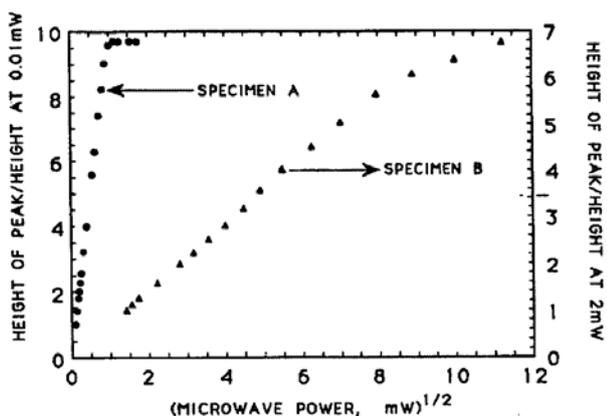
Figure 10. The ESR signal intensity of the specimens as function of microwave power showing the saturation.
