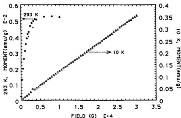
Figure 1. The magnetisation of the Specimen A expressed as the magnetisation per gram in emu as a function of applied magnetic field at 293 K and at 10 K.
