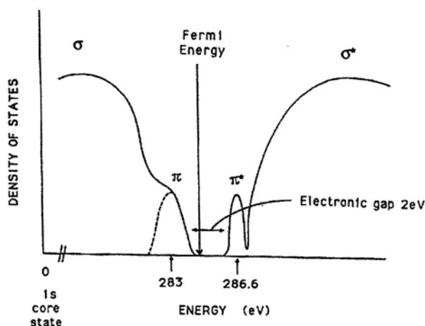
Figure 11. A schematic diagram of the density of states for ta-C showing the states labelled  $\pi$  and  $\pi^*$  arising from  $sp^2$  bonded atoms and states labelled  $\sigma$  and  $\sigma^*$  arising from  $sp^2$  and  $sp^3$  bonded atoms.
