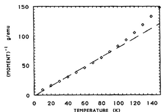
Figure 6. The reciprocal of the paramagnetic part of the magnetisation of the Specimen A at  $10^4$  Gauss as a function of temperature. The Curie-Weiss relation is well obeyed at low temperatures.
