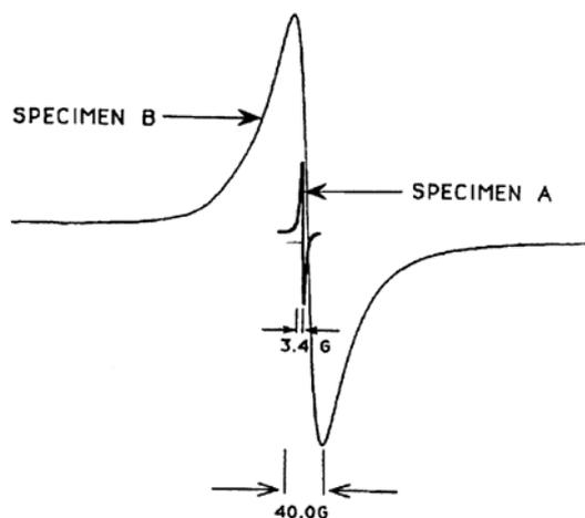
**Figure 7.** The first derivative of the electron spin resonance absorption in the Specimen A (small narrow signal) compared with that of the Specimen B (large broad signal).
