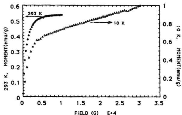
Figure 2. The magnetisation as a function of applied magnetic field for the Specimen B at 293 K and at 10 K.
