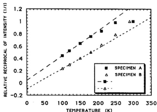
**Figure 8.** The reciprocal of the ESR signal intensity for the Specimen A (solid symbols) and the Specimen B (hollow symbols) in arbitrary units as a function of temperature. Except for temperatures above room temperature a Curie-Weiss law is obeyed approximately.
