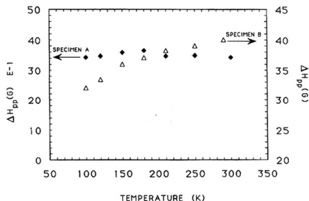
**Figure 9.** The linewidth of the ESR signals of the Specimen A and the Specimen B as a function of temperature.
