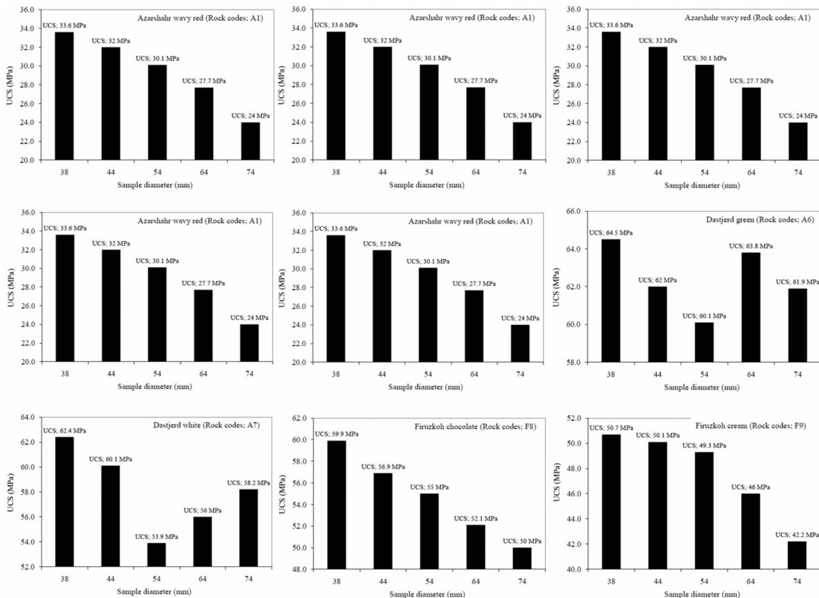
Figure 4. Uniaxial compressive strength versus specimens' diameter.
