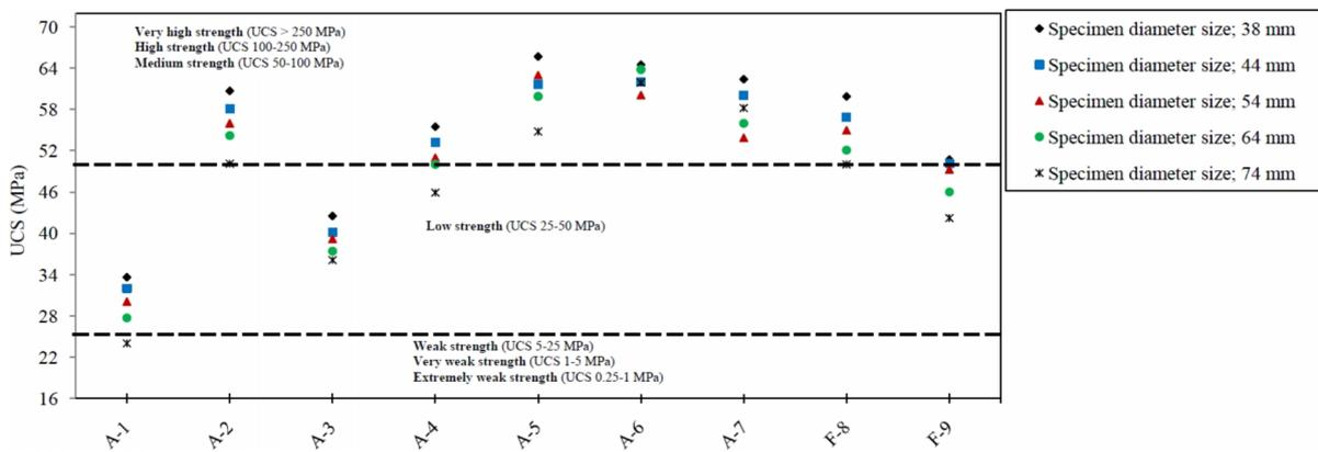
Figure 7. Samples classification based on UCS by ISRM [10] at different diameter sizes.
