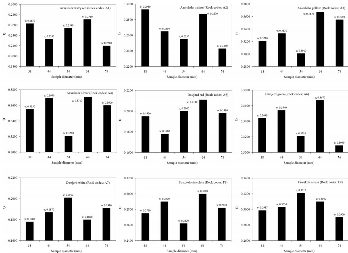
Figure 6. Poisson's ratio versus specimens' diameter.
