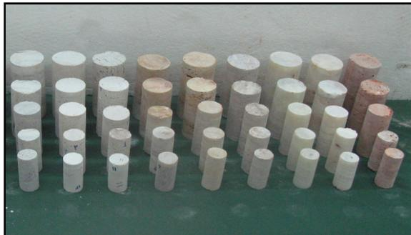
**Figure 2.** Core samples at five different diameters.
