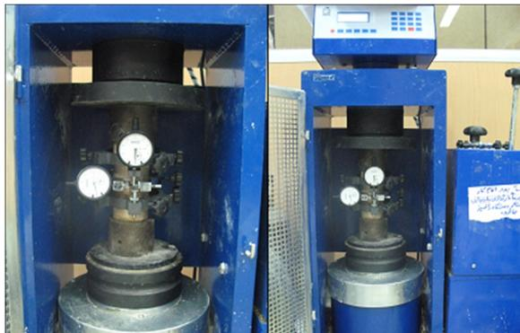
**Figure 3.** Uniaxial compressive strength apparatus for determination of UCS, E and  $\nu$ .
