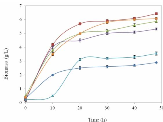
**Figure 2.** Effect of different carbon sources on the biomass of *A. eutrophus* in Arabinose (♦), Fructose (●), sucrose (\*), lactic acid (×), lactose (▲), Glucose (■).
