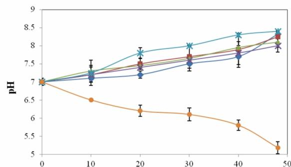
**Figure 8.** pH changes for different nitrogen sources during 48 h. Yeast extract (▲), Peptone (◆), Tryptone (■), Ammonium chloride (●), Urea (\*), Ammonium sulfate (×).
