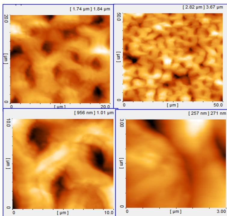
**Figure 10.** AFM topographic images of PHB films. Scan sizes are shown on top of each picture. The rough surface of fresh-prepared sample (exposed to air) is seen.
