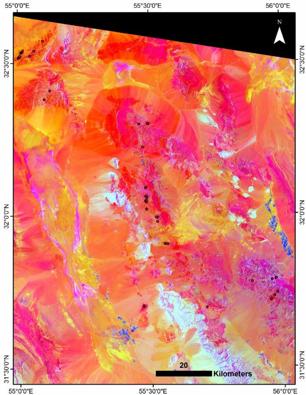
**Figure 4.** Landsat ETM<sup>+</sup> ratio image (bands 3/4, 5, and 5/7 in red, green, and blue, respectively) for the study area, showing the altered rocks as pale pink. The anomalies (red circles) are mainly located in the altered areas. Altered areas coincide with mountainous areas and show a remarkable decrease towards the northwest of the image.
