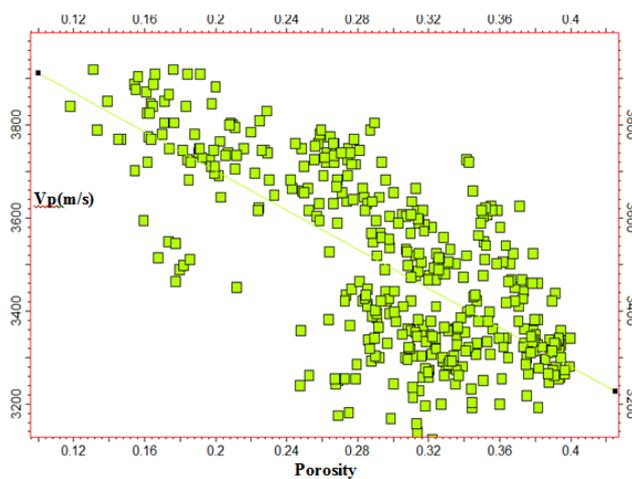
**Figure 7.** Crossplot of P-Velocity against Porosity from Tamag-4 Well within Reservoir Sand B Interval Indicating a Constant Cement Model Trend.
