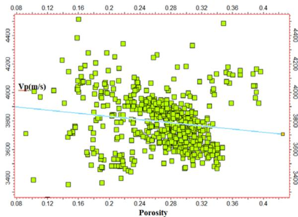
**Figure 6.** Crossplot of P-Velocity against Porosity from the Uppermost Part of Tamag-4 Well within Reservoir Sand A Interval indicating a Friable Sand Model Trend.
