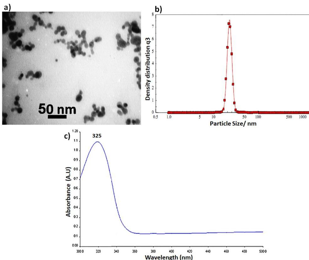
**Figure 2.** a) Representative TEM image and b) DLS and c) UV-visible spectra of Ag/Cs/PLG/CPS NPs .
