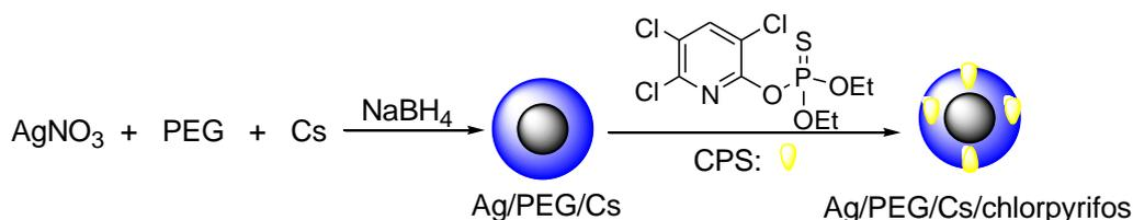
**Figure 1.** The schematic representation of Ag/Cs/PEG/CPS NPs synthesized from  $\text{AgNO}_3$  by reduction method.
