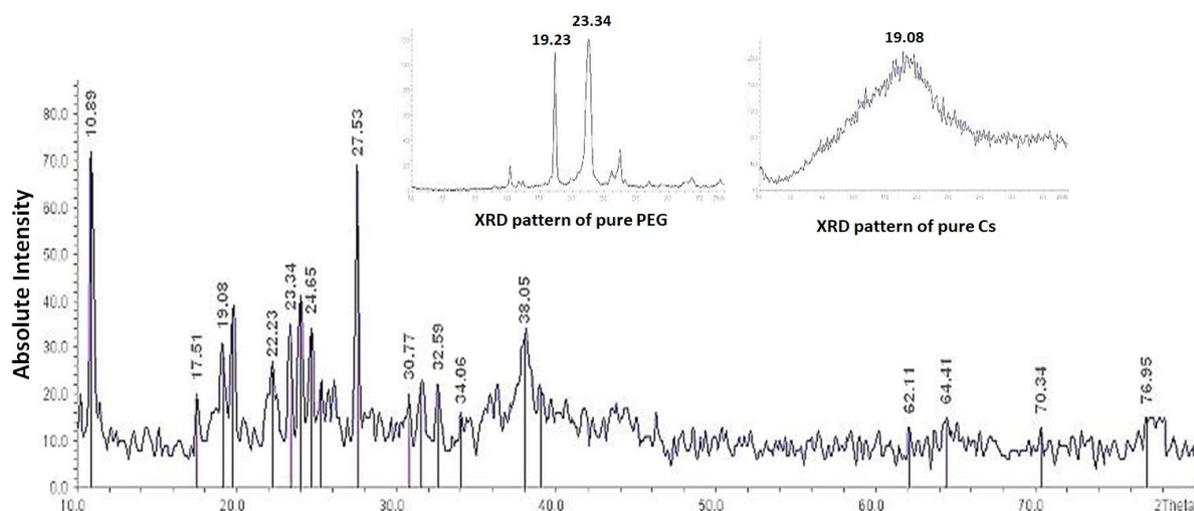
**Figure 4.** The powder XRD pattern of Ag/Cs/PEG/CPS NP. The inset images are related to the pure PEG and pure Cs.
