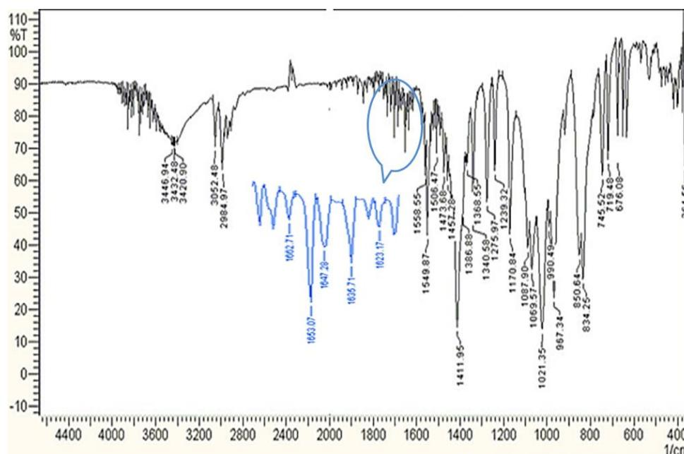
**Figure 3.** FT-IR spectrum of Ag/Cs/PLG/CPSNPs, the inset is related to the expanded part in the region of  $1690\text{-}1615\text{ cm}^{-1}$
