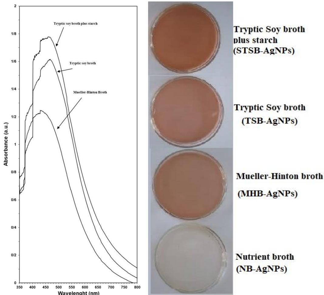
**Figure 1.** Left illustration demonstrates UV-vis spectra recorded after the addition of different culture supernatants of *K. pneumoniae* grown in tested culture media (1 ml) to silver nitrate organic solution (1 mM; 100 ml) and allowed to stand for 5 min in bright condition under visible light irradiation ( $1000 \text{ mmol}/\text{m}^2 \text{ s}$ ). Right illustration shows the test petri-dish containing the AgNPs samples prepared in acetone-water mixtures.
