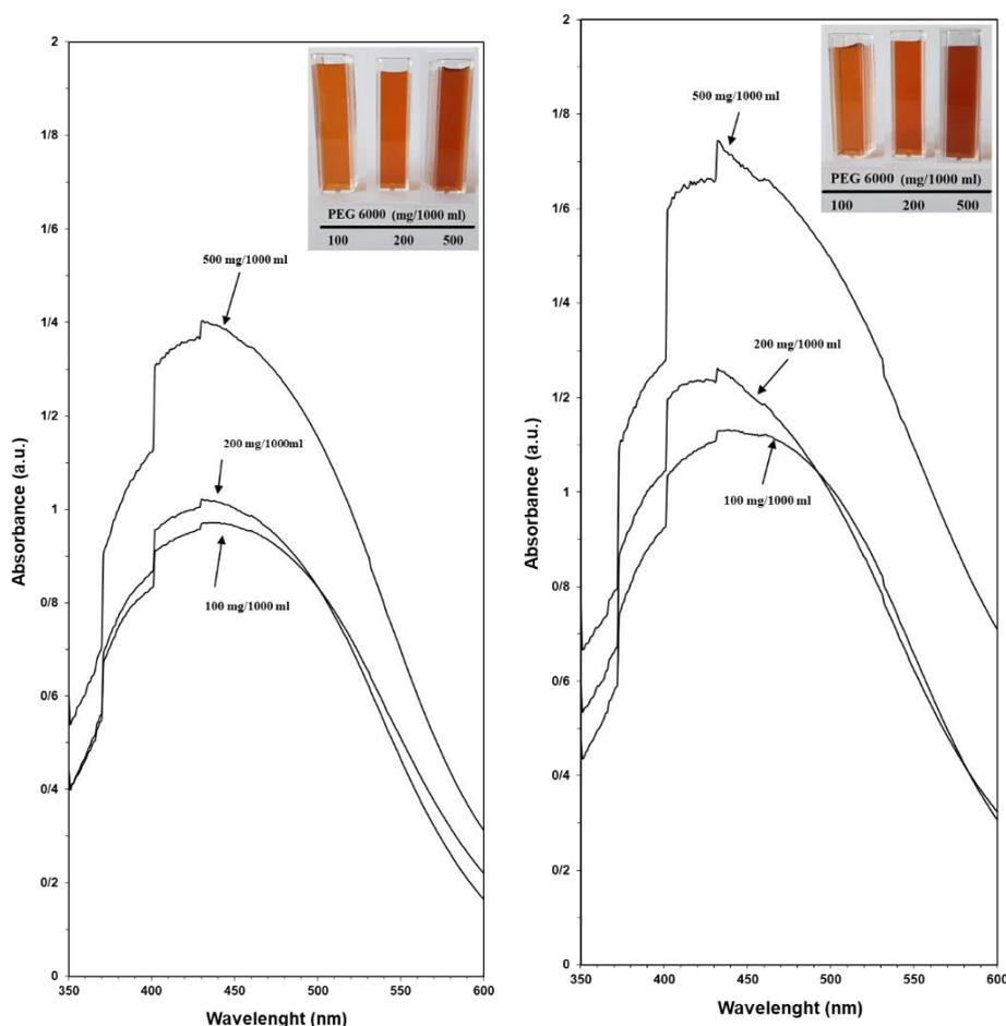
**Figure 2.** UV-vis spectra of STSB-AgNPs colloids. Spectra recorded after re-dispersion of different tested dry AgNPs concentrates in distilled water before (left illustration) and after (right illustration) treatment in ultra-sound sonicator bath for 6 min. The insets in the left and right illustrations show the cuvettes containing the different STSB-AgNPs colloids before and after sonication procedure.
