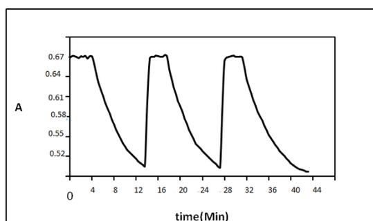
**Figure 4.** The response profile for the structured optode versus repetitive change in the concentration of Ag<sup>+</sup> cation from 0 to 10<sup>-5</sup> M and vice versa. The solution pH was adjusted at 6.
