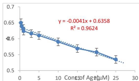
**Figure 5. b)** The calibration graph for the Ag<sup>+</sup> cation in the concentration range of 10<sup>-6</sup> – 2.5×10<sup>-5</sup> M at pH 6.
