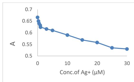
**Figure 5. a)** The response graph for Ag<sup>+</sup> cation in the concentration range of 0 to 30 μM at pH 6
