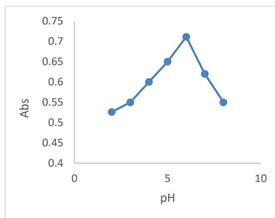
**Figure 2.** The influence of pH on the absorbance of a typical membrane. The concentration of Ag<sup>+</sup> cation in all tests was 10<sup>-5</sup>M.
