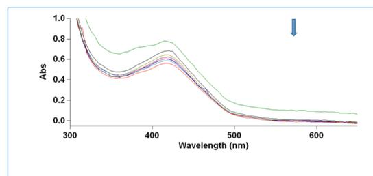
**Figure 6.** The Absorbance spectra of Ag-TY complex in immobilized form of the concentrations of Ag<sup>+</sup> cation, being the same as the concentrations, presented in the figure 5a. The arrow in the figure indicates the increasing direction of the concentration of Ag<sup>+</sup> cation in the solutions.
